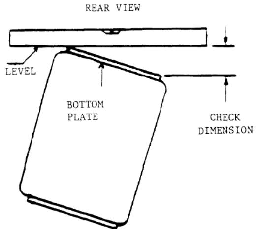
Record Check Dimension as Twist \_\_\_\_\_
